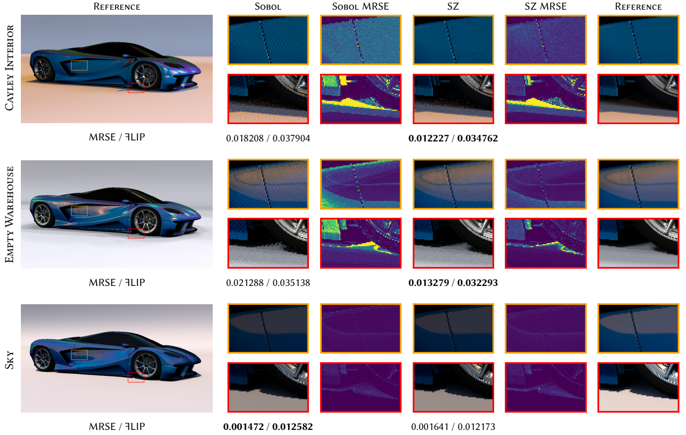
Fig. S1. Comparisons of images rendered using the Sobol sequence and using our SZ sequence. All images are rendered with 64spp with direct lighting only, using four varied environment maps. Crops show representative results; full images are available in our supplemental material. See Figure S2 for the specification of the heatmap used to visualize MRSE error.
