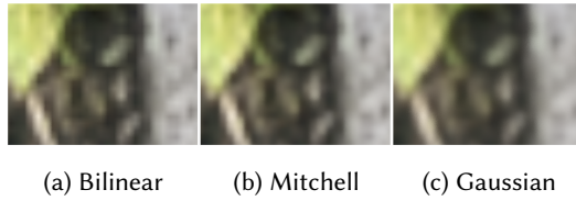
Fig. 10. Bilinear filtering (a) compared to stochastic, single sample estimation of the bicubic Mitchell (b) and Gaussian (c) filters, resolved with DLSS’s temporal accumulation. The Mitchell filter is much sharper than the bilinear and does not produce diamond-like artifacts. The Gaussian filter is isotropic and although it tends to blur textures, it gives the best results for reconstruction of diagonal lines.
