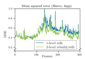
**Figure 7:** Error over time for an animation of the Bistro scene rendered at 4 spp. The benefit of rebuilding the top-level BVH results in an up to 1.4× reduction in MSE compared to using a one-level BVH that is refitted every frame. Notice that locally the differences can be much larger; see Figure 8.
