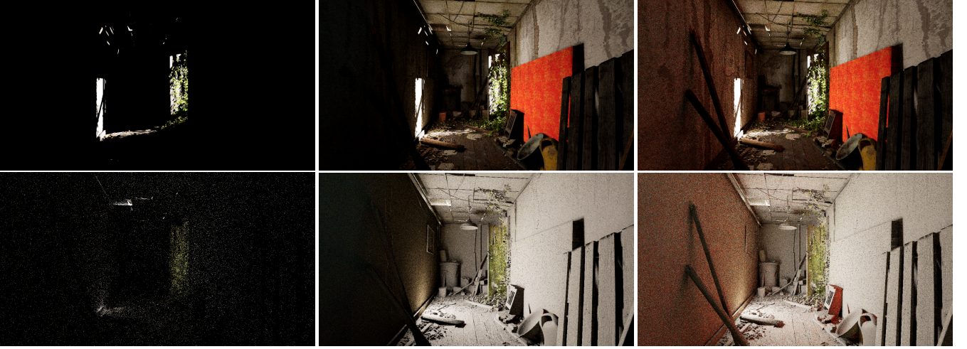
Figure 8: Comparison between direct light, 1-bounce and 2-bounce GI rendered with our algorithm. Top row, left to right: scene rendered with direct lighting, one-bounce, and two-bounce global illumination. Bottom row: the indirect illumination alone, left to right: two-bounce path tracing, one-bounce, and two-bounce ReSTIR GI result. Rendered at 1920 \times 1050 resolution on an NVIDIA RTX 3080 GPU, for ReSTIR GI, initial sampling takes 3.2 ms for one bounce and 4.2 ms for two. Sample reuse uses 4.6 ms in both cases. The 2-bounce path tracing takes 6.9 ms.
